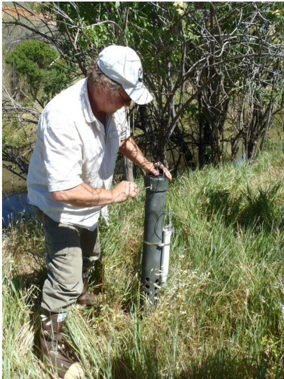
deploying the continuous water quality monitor
